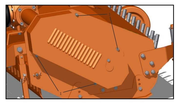
Apply a force of about 10-15 kg on the middle of the belts set, and measure the entity of the consequent deflection of the belts (see picture):
