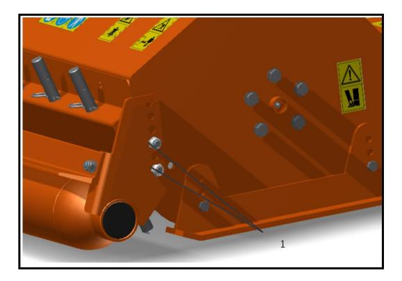
Depending on the different roller positions, it is possible to set four different cutting heights: 32-57-82 and 107 mm.
