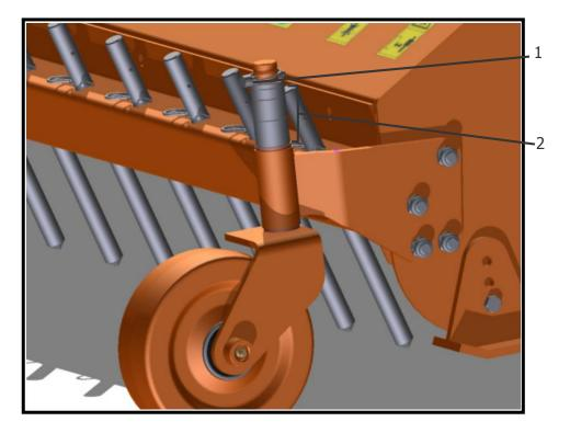
Depending on the different position of the spacers on the shaft, it is possible to set fivedifferent cutting heights: 70-76-89-114 and 145 mm.
