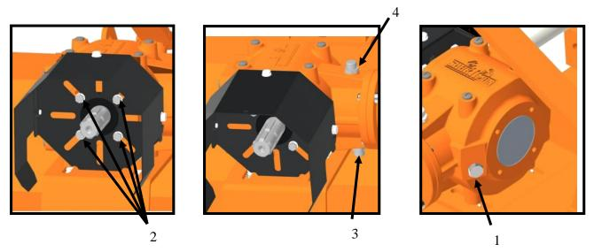
If the oil level is below the line of the level plug, it's necessary fillup oil till restore the correct level.
